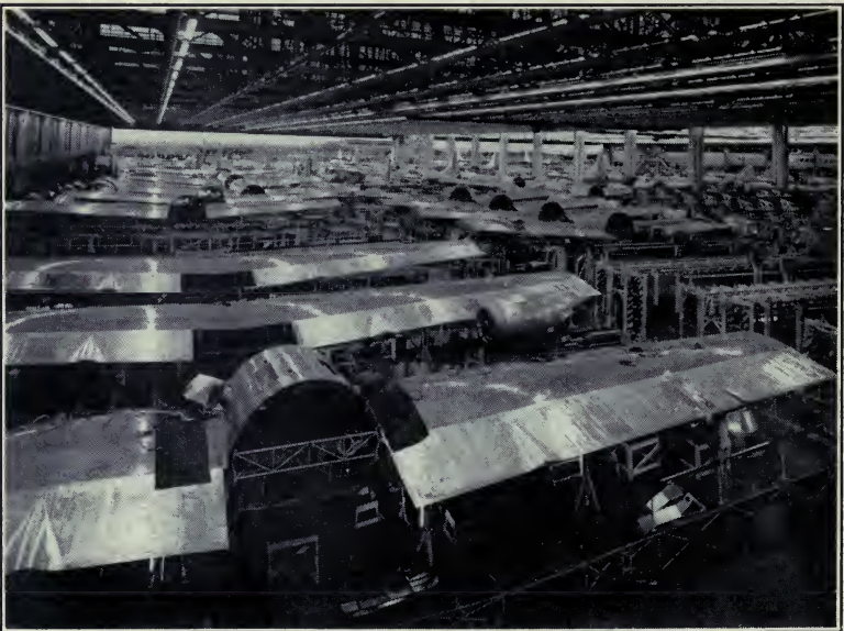
Wing Sections in the Assembly Area of the Boeing Wichita Plant.
