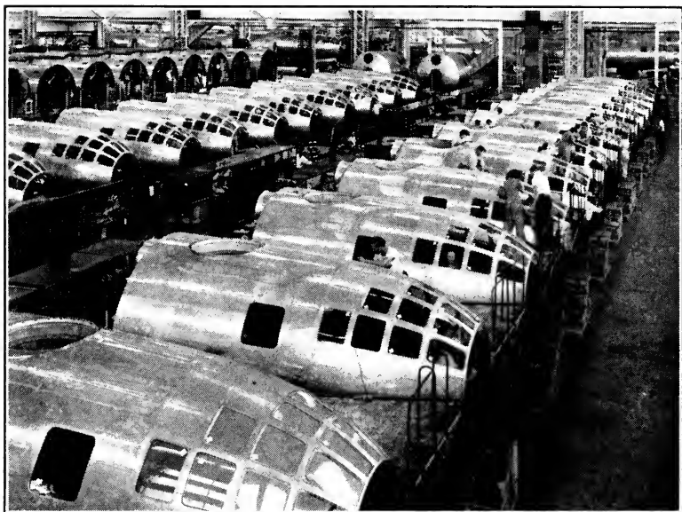
Nose Sections, and in the Left Background the Double Bomb Bay Sections.
