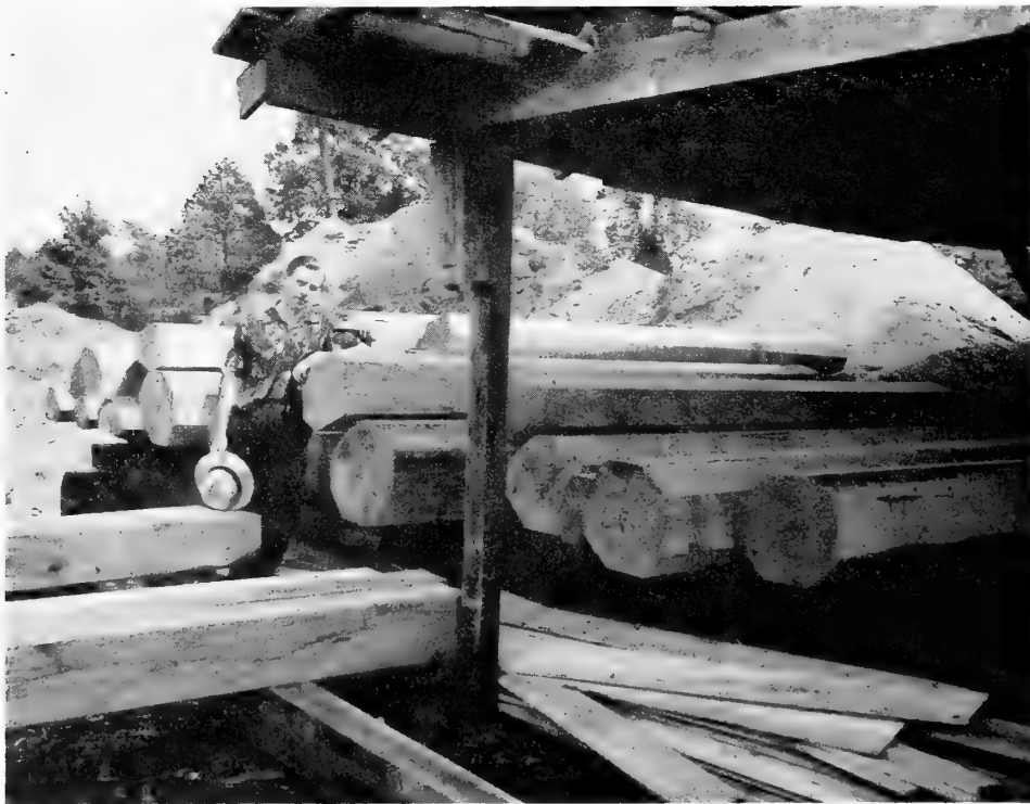
FIGURE 34.—Red oak veneer flitches at a sawmill in Allen County. They have been carefully sawed from high-quality logs and will be shipped to a veneer mill for further manufacture.
