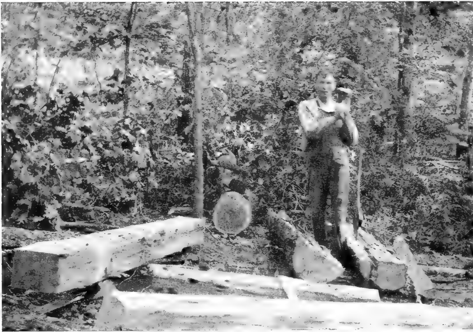
FIGURE 36.— Hewing crossties is a slack-time job for people living within the forest. The ties are usually hewn from small sawtimber and few tools are needed.
