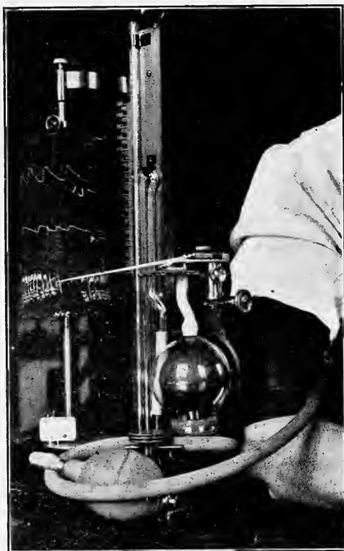
FIG. 189.—Erlanger's Sphygmomanometer. Shown with the Rubber Bag Attached to the Arm. The picture is taken at the end of an experiment after the pressure in the instrument is run up again to above the systolic pressure. The upper part of the cylinder shows a sphygmogram taken with the instrument. (Experiment and photo by Hill and Watkins.)
