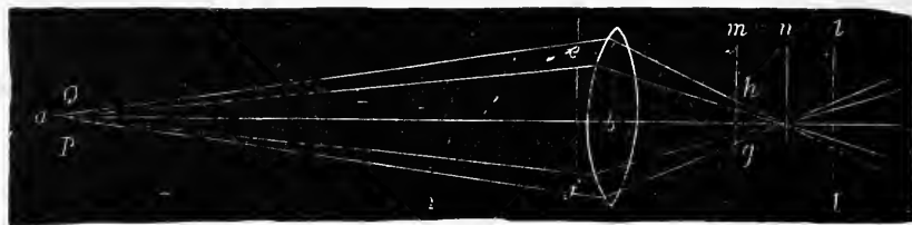
FIG. 482.—Diagram of Experiment to Ascertain the Minimum Distance of Distinct Vision.
