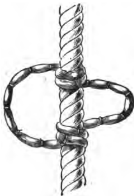
Fig. 125.—Selvagee fastening Block to Rope.
