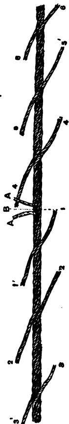
Fig. 186.— Long Splice, all Ends ready for Tucking.
