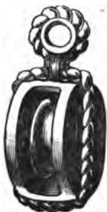
Fig. 138.—Stropping a Block.
