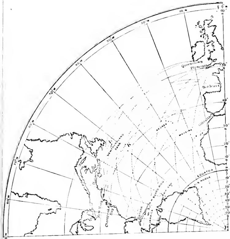
QUARTER OF THE SOUTHERN CHART on the same Projection (and on the same scale), showing fourteen illustrative great circle tracks in the North Atlantic, obtained by the same method. [L and K mark the points where the steamships from Queenstown and from Bordeaux respectively cross the Newfoundland Bank.]
