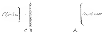
FIG. 2.—The "Eye-lenses," B, act as Telescopes. Aerial foci at A and C.
