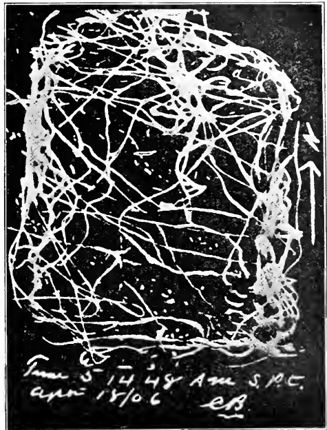
Signature of the San Francisco Earthquake. Written by means of the seismograph at Oakland, California.
