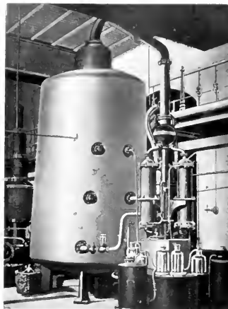
FIGURE 484. A huge still of fifty thousand gallons capacity.
