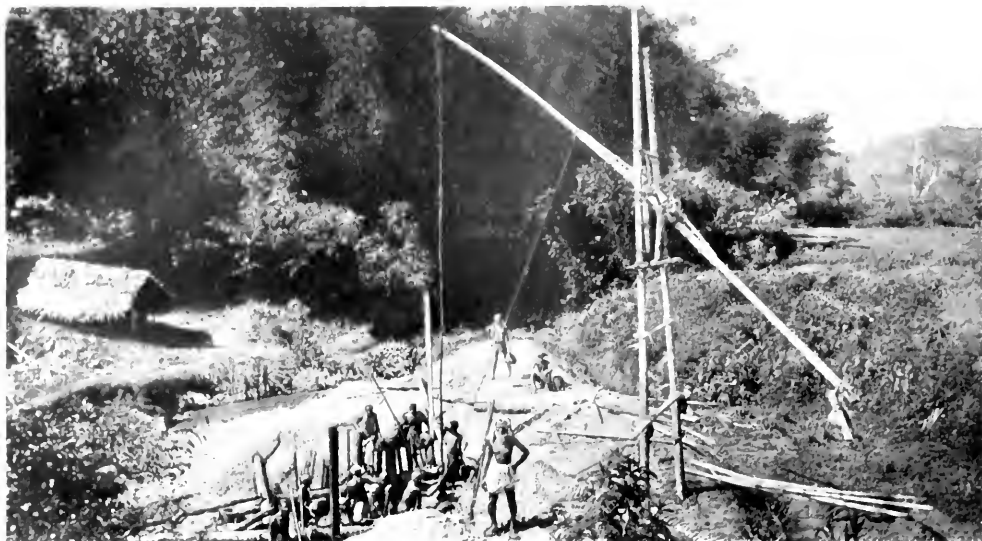
FIGURE 1. Gem pit showing primitive crane and pool at which the earth is washed for gems.
