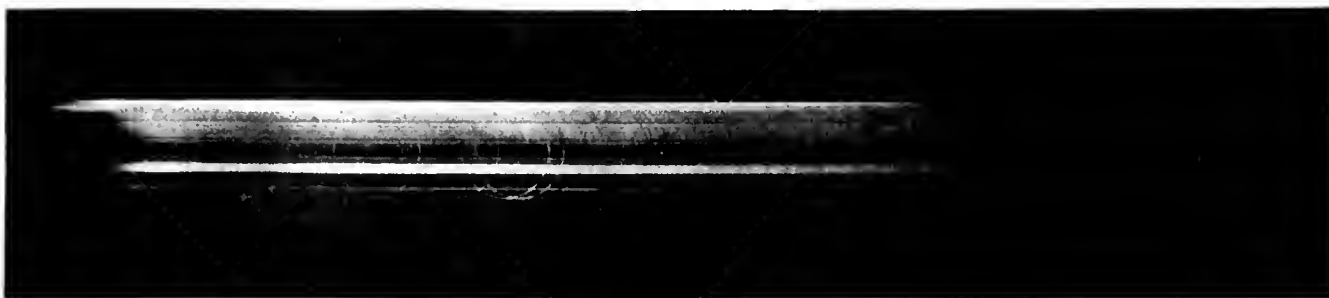
From a photograph by J. H. Worthington. FIGURE 521. Flash spectrum obtained near Ovar, Portugal, 1912, April 17th, during a total solar eclipse, with a prismatic camera consisting of a 2.1 inch Achromatic Quartz and Rock-salt lens of 50 inches focus with two 50 Quartz prisms in front of it. Exposure, about \frac{1}{4} -second. The photograph from which this is taken is unique. (See "KNOWLEDGE," November, 1913, page 408.)
