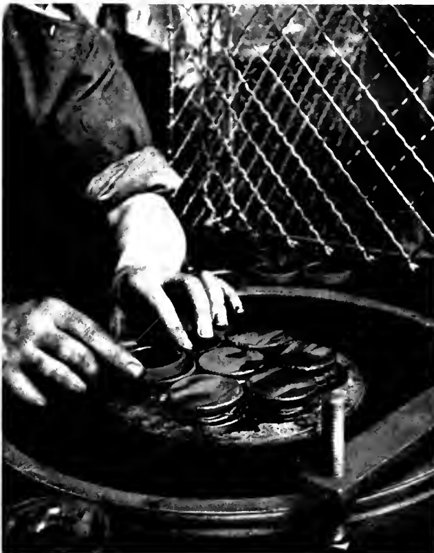
FIGURE 257. Testing a lens with a proof plate.
