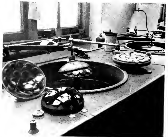
FIGURE 255. Lens polishing machine with blocks of lenses.
