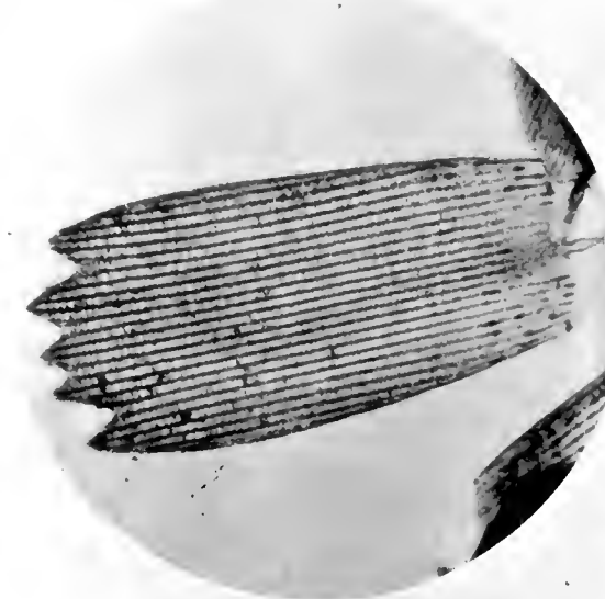
FIGURE 97. The same scale taken by Swift & Son's new two-thirds inch apochromatic objective of 0.30 N.A. Magnified four hundred and seventy diameters, as before.
