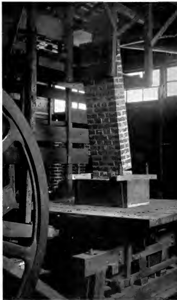
FIGURE 158. "Shaking Table" in the Seismological Institute, Tokyo University. The bricks are made specially for testing purposes from brick columns previously destroyed by earthquake. They are pulled asunder in order to find out the strength of the brick and mortar joint.
