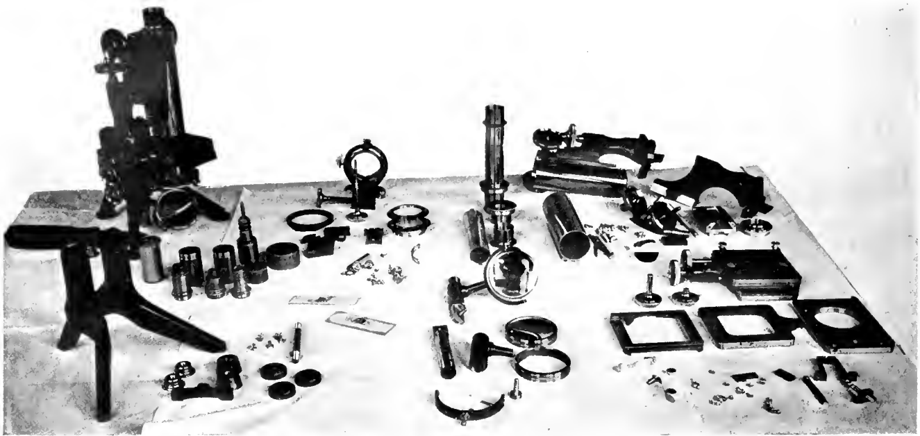
FIGURE 262. A microscope stand (H Edinburgh Student's) with its components and their individual pieces.
