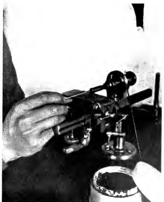
FIGURE 259. Grinding the edge of a lens for a one-twelfth objective.
