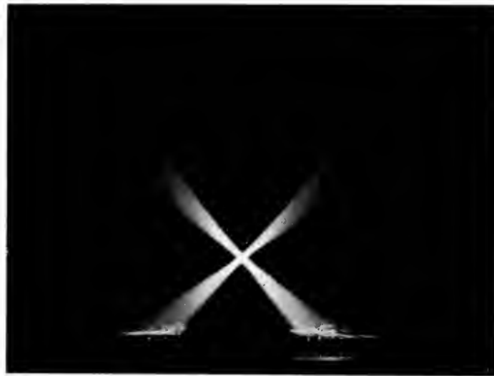
FIGURE 276. The intersecting pencils of light within fluorescent uranium glass.
