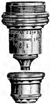
FIGURE 275. An objective with the nickel-plated part unscrewed.
