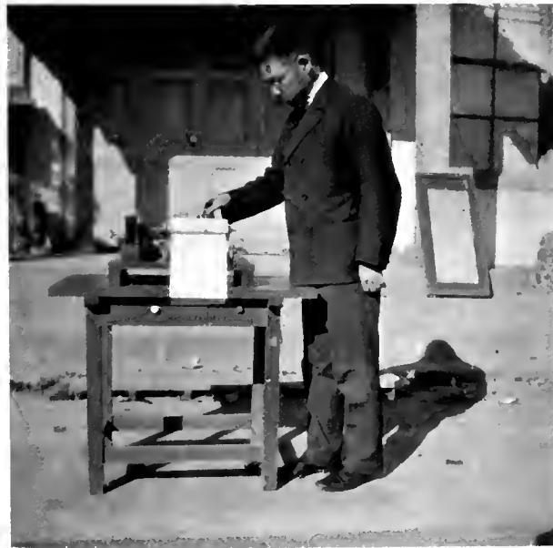
FIGURE 157. Professor Omori with Vibrating Recorder at the Seismological Institute, Tokyo. By means of this instrument vibrations of railway bridges and steamers are measured.
