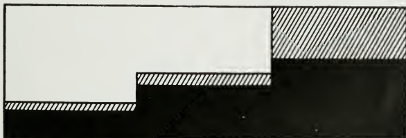
SHADOWS HALFTONES HIGHLIGHTS Showing that a Flattening Reducer removes more silver from the dense than from the thin parts of a negative
