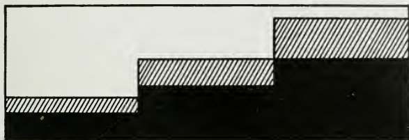
SHADOWS HALFTONES HIGHLIGHTS Showing that the same percentage of silver is removed from all the tones by a Proportional Reducer
