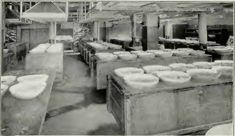
Illustration No. 3—DISSOLVING BARS OF SILVER TO FORM SILVER NITRATE
