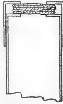
FIG. 17.—DIAPHANOSCOPE, WITH LEAF DISCS IN POSITION, IN LONGITUDINAL SECTION; \times \frac{1}{2} .
