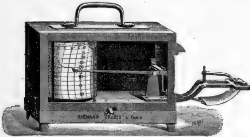
FIG. 46.—THE RICHARD THERMOGRAPH; \times \frac{1}{2} .
