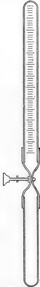
FIG. 25.—REAGENT (LOWER) AND GRADUATED TUBES, WITH RUBBER CONNECTION AND CLAMP; \times \frac{3}{4} .
