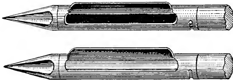
FIG. 56.—Fränkel's instrument for obtaining earth from various depths for bacteriologic examination.
