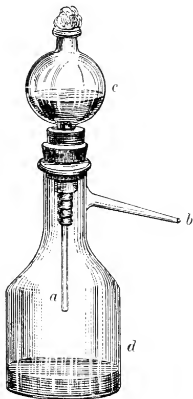
FIG. 22.—Kitasato's filter: a , porcelain bougie; b , attachment for suction-pump; c , reservoir; d , sterile receiver.
