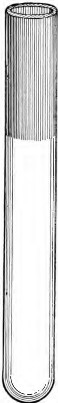
FIG. 29.—Providence Health Department tube of heavy glass, with etched surface for writing data. These tubes are etched by dipping for thirty seconds in "white acid."
