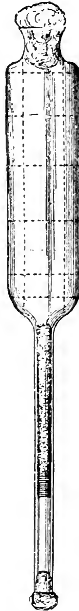
FIG. 55.—Sedgwick's expanded tube for air examination.
