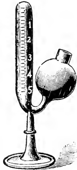
FIG. 32.—A graduated fermentation-tube.
