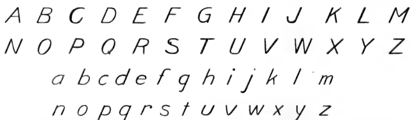
FIG. 1.—The alphabet in suitable style for free-hand lettering.
