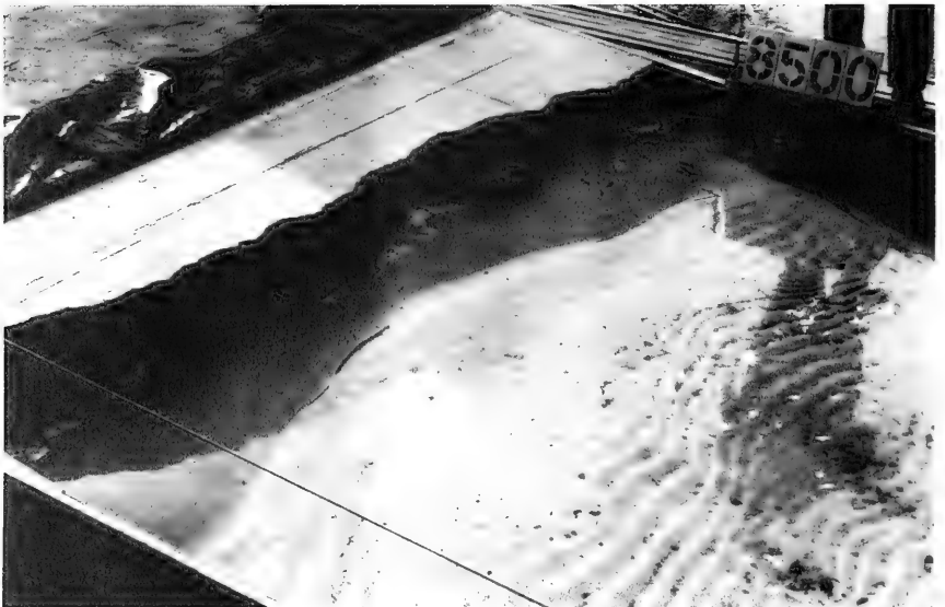
b. At 85 hr Figure 36. Foreshore variability over 35-hour period in experiment 72C-10 ( L/W = 1.03 ).
