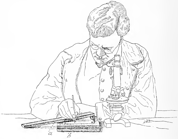
FIG. 1.—Illustrating the use of the drawing-board, b , and hand-rest, a , and the proper position for a right-handed person when drawing microscopical preparations. The raised end of the hand-rest a , is placed upon the drawing-board b , and its other end allowed to rest on the table.
