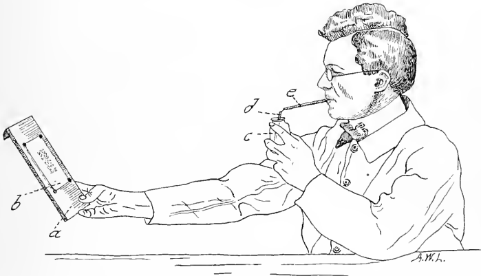
FIG. 14.—Illustrating use of apparatus and position assumed in “fixing” a drawing.
