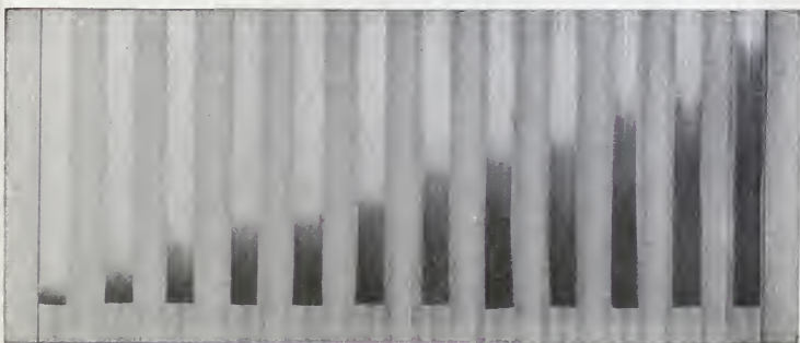
2 5 10 15 20 25 30 35 40 50 60 70 FIG. 22b.—Standard Arsenic Bands in Micromilligrams of As_2O_3 (Ammonia Development).
