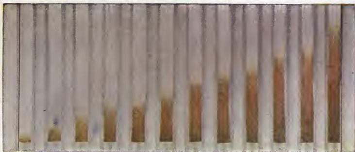
2 5 10 15 20 25 30 35 40 50 60 70 FIG. 22a.—Standard Arsenic Bands in Micromilligrams of As_2O_3 (Hydrochloric Acid Development).
