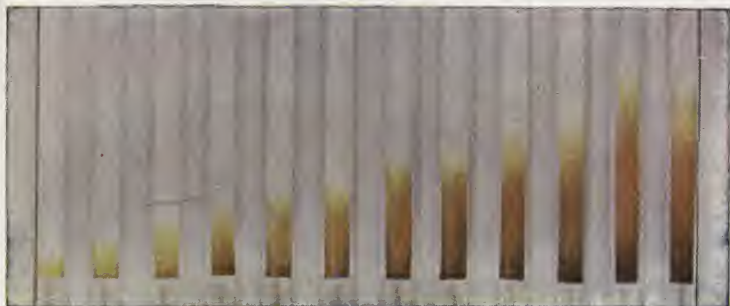
2 5 10 15 20 25 30 35 40 50 60 70 FIG. 22.—Standard Arsenic Bands in Micromilligrams of As_2O_3 (Initial).
