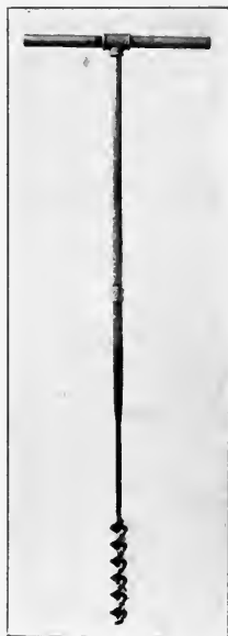
FIG. 1. — A soil auger made by welding a \frac{3}{8} -inch gas pipe to a 1\frac{1}{4} -inch wood auger.
