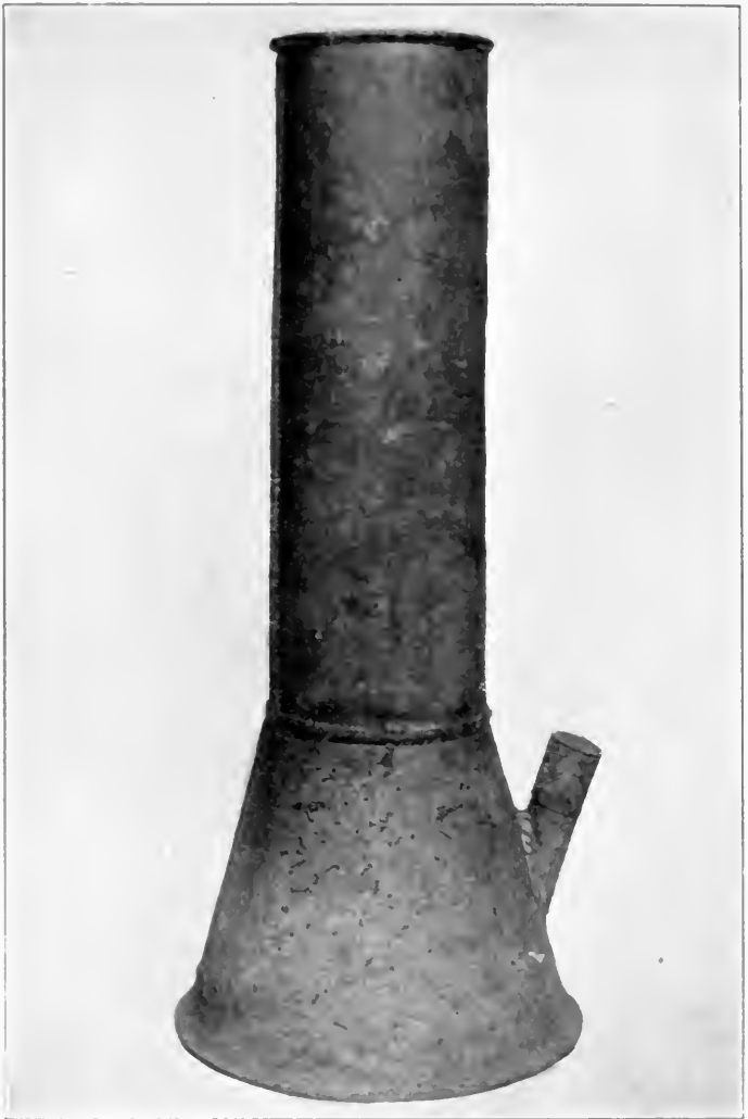
FIG. 4.—A cylinder suitable for demonstrating the effect of mulches on evaporation of water from soils. Made of galvanized iron. Dimensions of cylinder eighteen inches long and four in diameter. The bottom of the cylinder is incased in a water jacket. The water in the jacket enters the soil by means of perforations near the bottom of cylinder.
