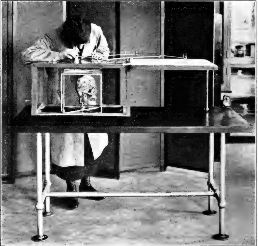
FIG. 14.—The dioptograph of Lucae in use. The operator is here following the contour lines of a skull as seen from the norma verticalis by means of the small telescope, and at the same time, by means of the attached pantograph, is sketching the same upon the sheet of drawing paper upon her left, mounted upon the drawing-board. As with other pantographs a skull may be thus drawn at a reduction or an enlargement, or can be drawn at exactly the natural size, as here.
