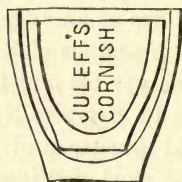
FIG. 27.—Copper assay crucible, in section.
