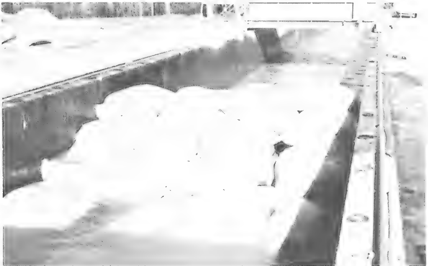
Figure 47. Backface after 50 waves shows shoreward row of bags across crest intact during wave condition a (test IV).
