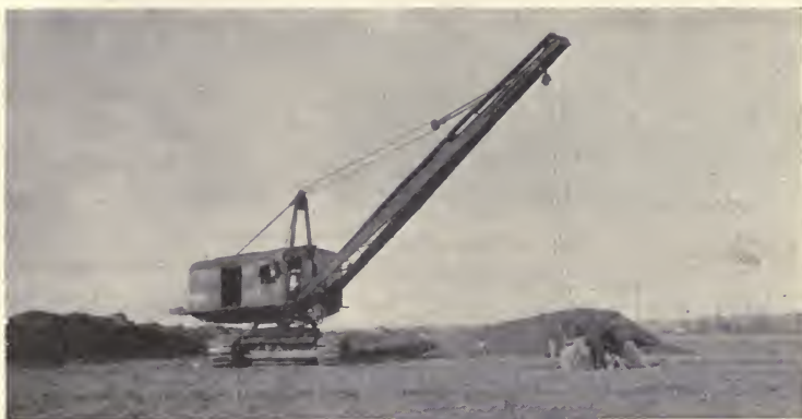
FIG. 62. Drag-line scraper excavator operated by electric power.
