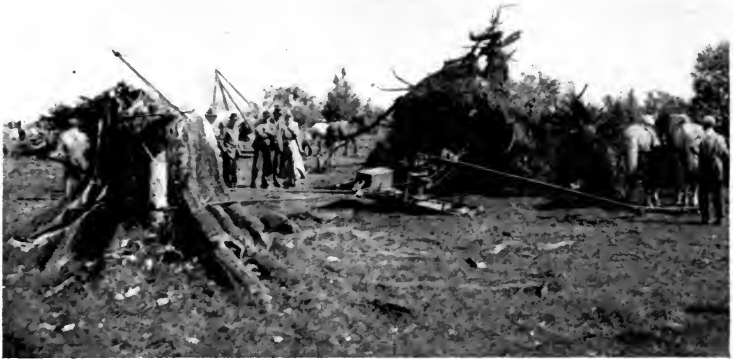
FIG. 44. A horse power puller in use. (Courtesy American Society of Agricultural Engineers.)
