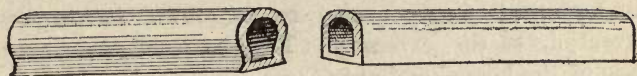
FIG. 8. HORSESHOE PIPE TILE, FIG. 9. FLAT-BOTTOMED PIPE TILE AFTER HENRY STEPHENS, 1848. AFTER FRENCH, 1859.
