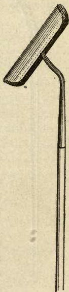
FIG. 30. MILES' DRAINING SCOOP.
