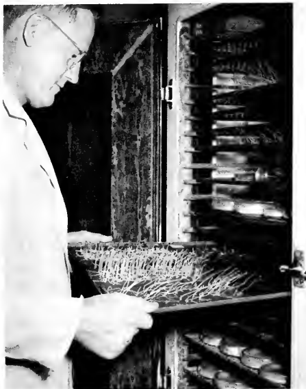
Checking germination of seeds on moist paper in a temperature-controlled chamber, during a germination test.
