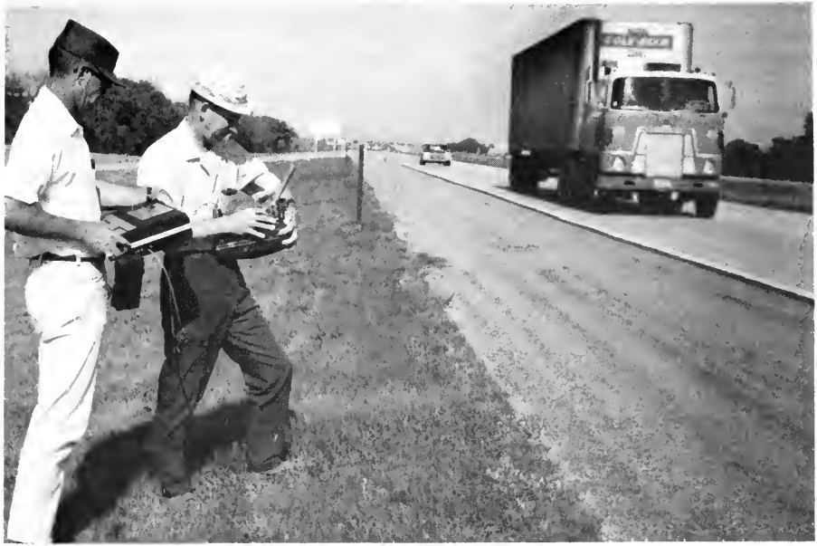
Scientists tape-record truck noise in preparation for studying the passage of sound through belts of trees and shrubs.
