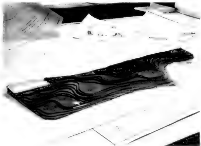
Fig 4.1 Egerton Gardens: cardboard model prepared as a design check.
