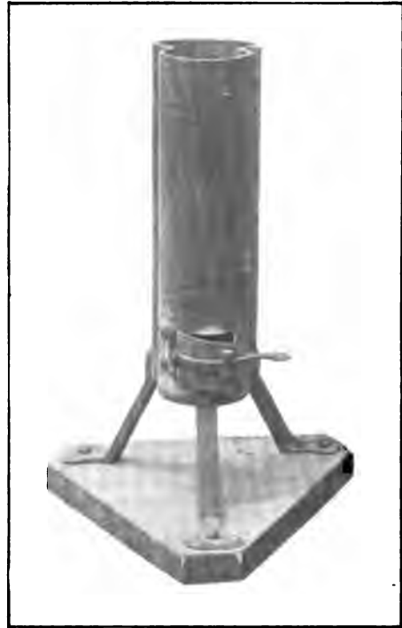
Fig. 54. — FOURNEAU A PLOYER.
