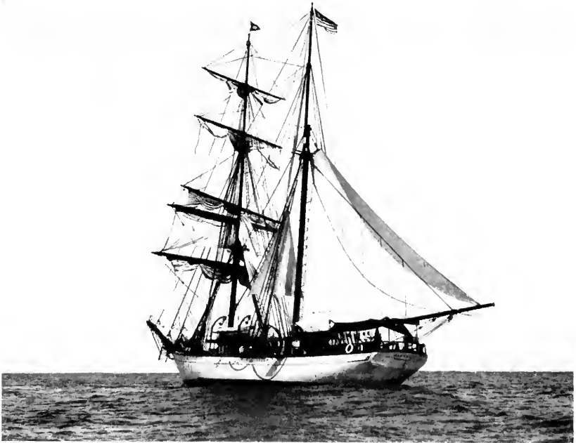
THE Carnegie HOVE-TO FOR AN OCEANOGRAPHIC STATION IN THE PACIFIC Only enough sail is carried to keep the ship headed into the wind.
