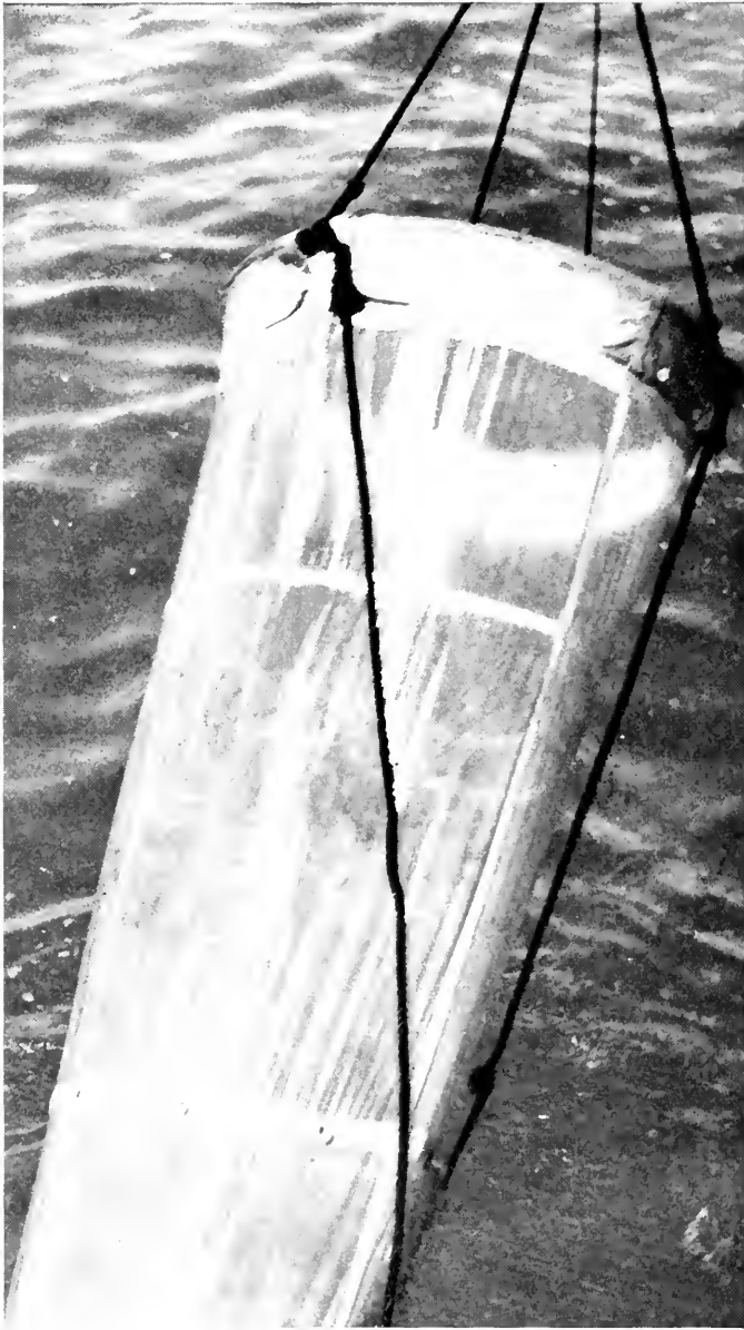
A SILK-NET COMING UP AFTER BEING TOWED FROM THE SHIP Used to collect the microscopic forms of life floating in the ocean.
