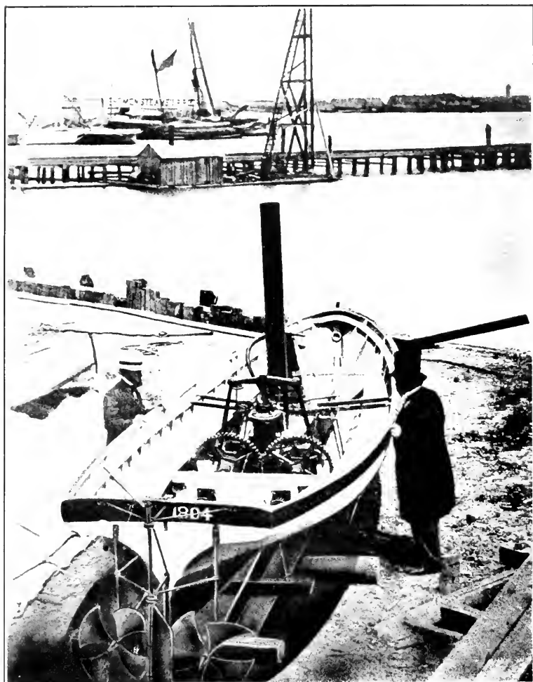
THE TWIN-SCREW PROPELLER OF 1804
