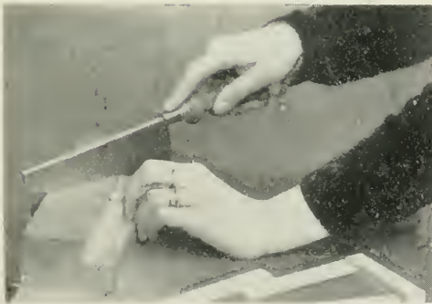
FIG. 28. OBLIQUE SAWING—ACROSS THE FIBRES.
