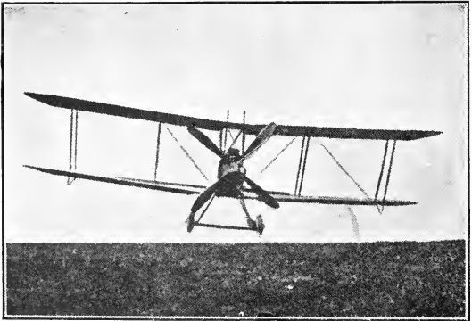
FIG. 36.—Bad landing Type 4—machine not level. Wheels do not touch ground at same time, and one may smash.
