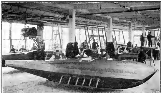
FIG. 14.—Building a flying boat hull. Note wing stumps and hydroplane fins.
