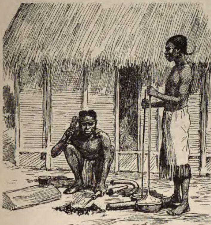
Forgeron Bayanzi. Soufflet double mu alternativement.
