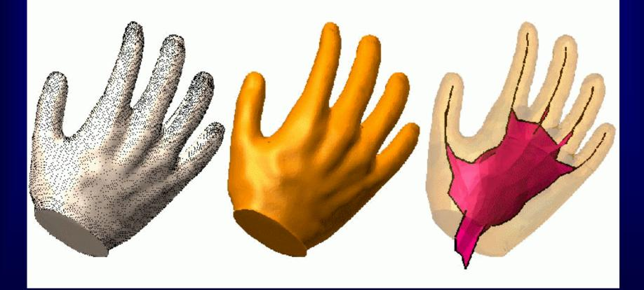
Laser range data, power crust, simplified approximate medial axis.
