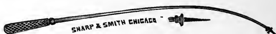
FIG. 83.—Rappaner's brush holder, one third size. The point is screwed into an ordinary camel's-hair brush, and the stem may be bent at any desired angle.
