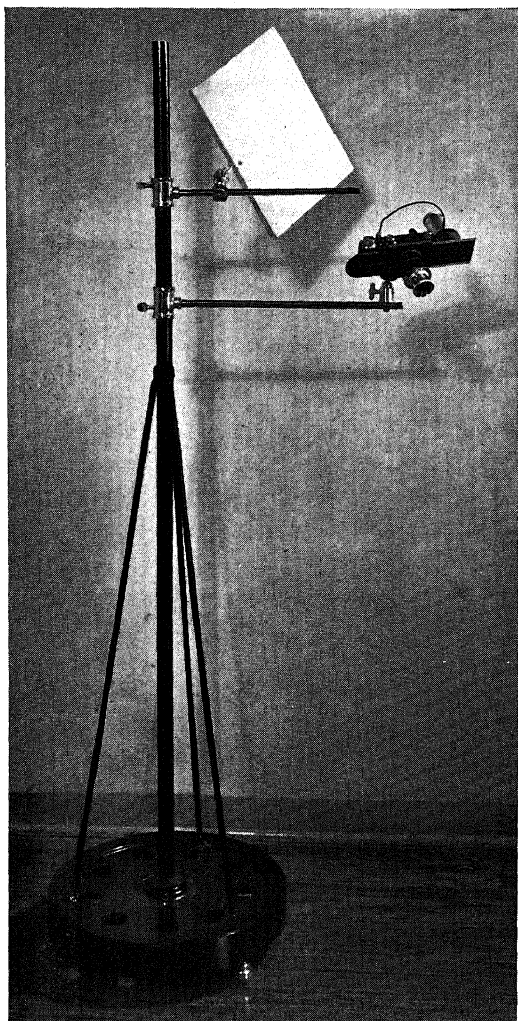
Fig. 333 Home-made Portable Camera Stand supporting Leica camera with Sliding Focusing Attachment and Reflector. The outfit is readily available for use at the dental chair. Both Camera and Reflector are easily adjustable, providing exceptional flexibility and rigidity.
