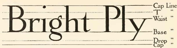
FIGURE 42. Diagram showing the ruling of guide lines for the construction of small letters
