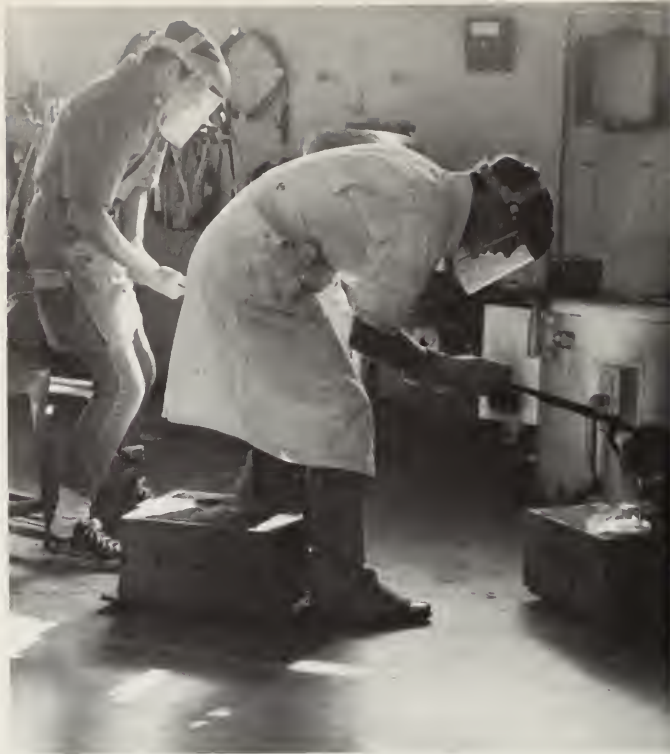
Steaming molten aluminum is poured into a sand mold by Mr. Frank Schmidt. Bill Hawkins aids his instructor while learning by doing
