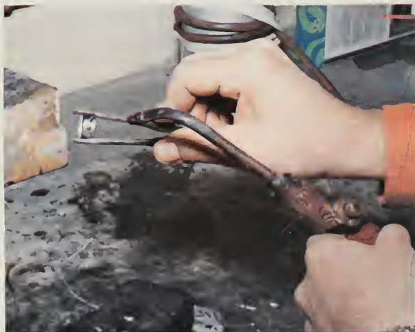
Shown here is a copper ring being soldered together. The ring has a second strip on the outside which forms the design.
