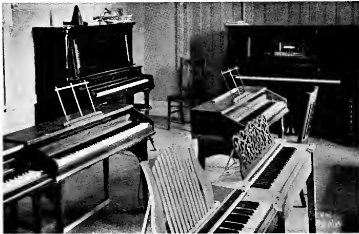
1933: THE ROSS MULTIPLE PIANO. It was patented by Prof. R. Wilson Ross of the music department. Its purpose was to enable a music teacher to instruct five or more students at one time with the "equal efficiency of the usual private lesson."
