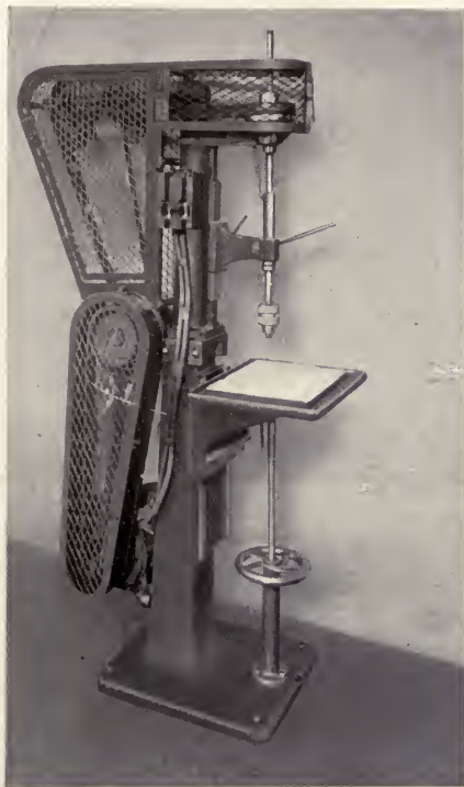
TYPE OF EXPANDED METAL GUARD USED ON DRILL PRESSES
