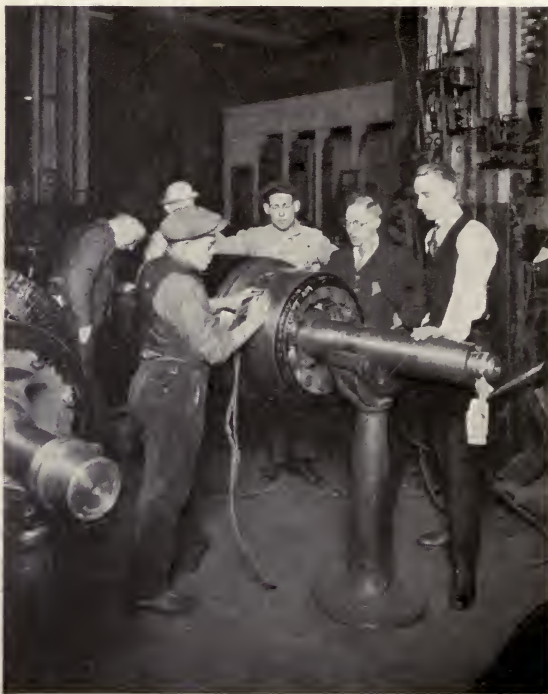
Fig. 85. LEARNING HOW TO TEST A MOTOR ARMATURE
