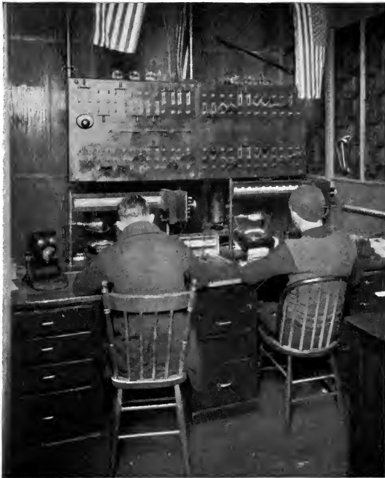
Fig. 84. MEASURING RESISTANCE OF INDUCTION MOTORS
