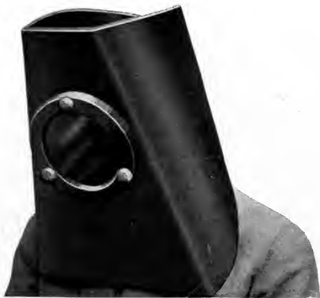
HELMET USED BY ARC WELDERS, PROVIDED WITH WINDOWS OF SPECIAL GLASS WHICH SHIELD THE OPERATOR NOT ONLY FROM INJURIOUS LIGHT RAYS BUT ALSO FROM THE HEAT RAYS
