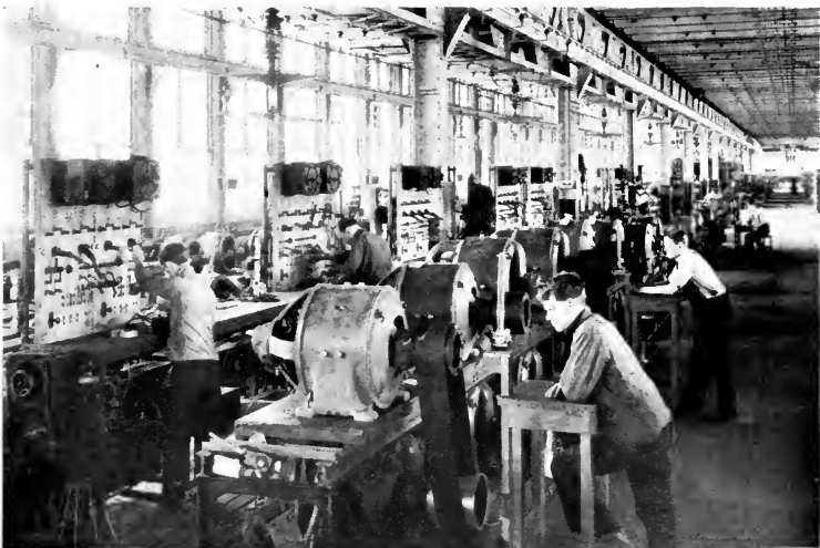
Fig. 83. COMMERCIAL TEST OF DIRECT-CURRENT MACHINES
