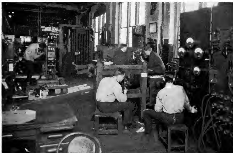
Fig. 88. TESTING SWITCHBOARD CIRCUIT BREAKERS AND RELAYS
