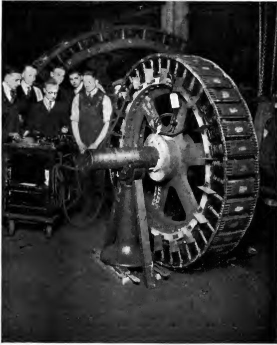
Fig. 86. INSTRUCTION IN TESTING ROTOR OF ALTERNATOR
