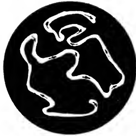
FIG. 65. TORTUOUS PATH OF A DROP OF HEAVY OIL (CHLOROFORM) ON A SHELLAC PLATE
