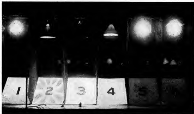
Comparison of various reflectors with tungsten lamps of the same size. 1. Opal shade; 2. Smooth aluminum reflector; 3. Reflector of pure silver; 4. Cone of blotting paper; 5. Bare lamp; 6. Flat mirror plate above lamp.
