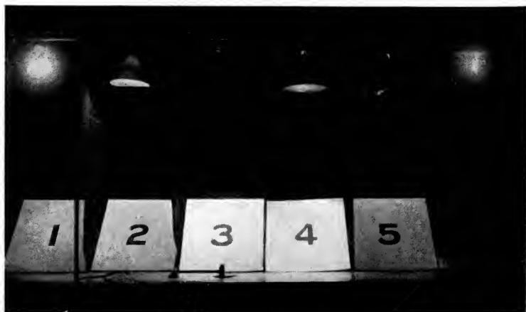
Comparison of their reflecting surfaces with tungsten and Welsbach lamps. 1. Welsbach inverted mantle opal shade; 2. Blotting paper; 3. Tungsten lamp in pure silver reflector; 4. Aluminum reflector over inverted gas mantle; 5. Ordinary newspaper; 6. A mirror plate.
