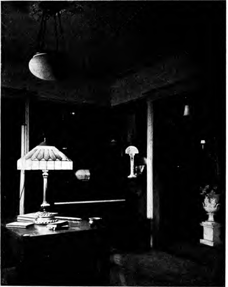
The table portable produces a homelike effect by leaving the walls in part shadow. This is an example of a good type of lamp, high pedestal and simple glassware.
