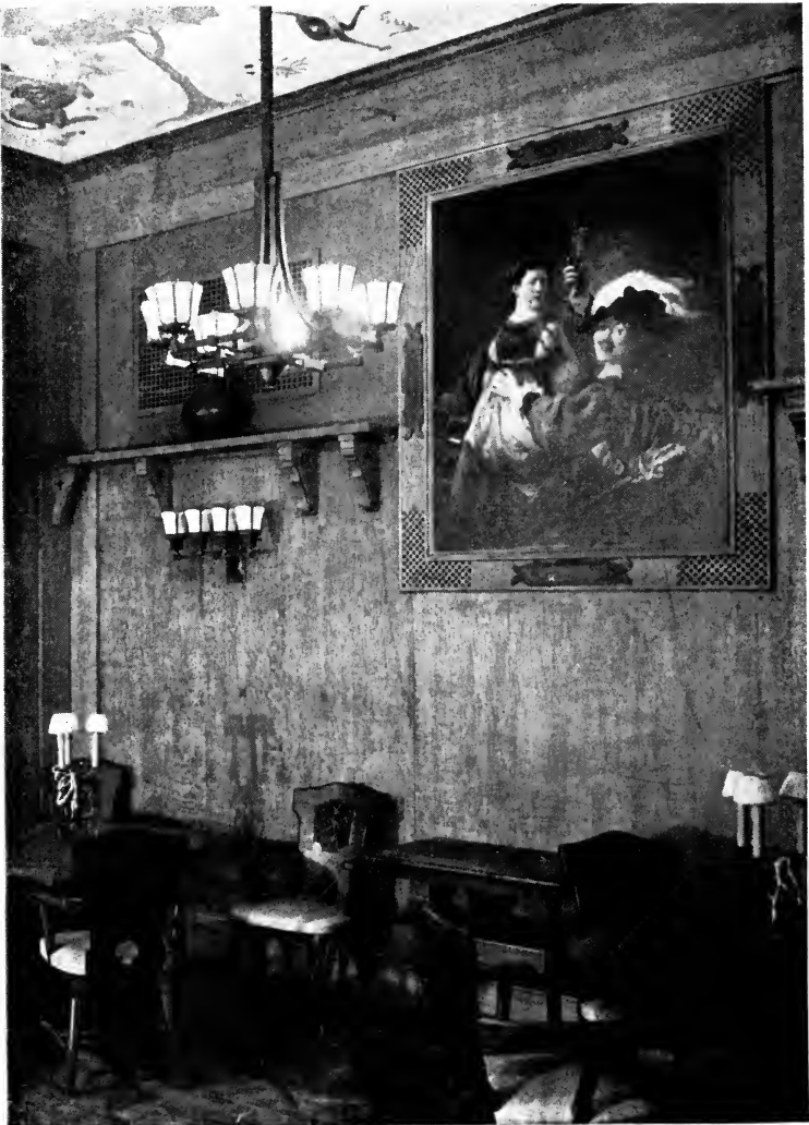
There is too much light here and it is wrongly placed. The lights hang too low and destroy all possible artistic expression of the picture. The lights against the wall are a source of glare.
