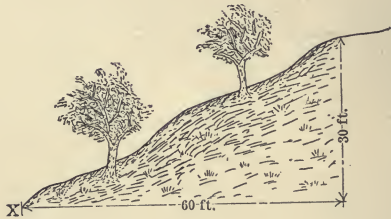
FIG. 3.—Effect of a hillside with a rise of one foot in every two.
