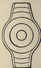
FIG. 28.—Glass brick, a block made for use in heavy walls.
