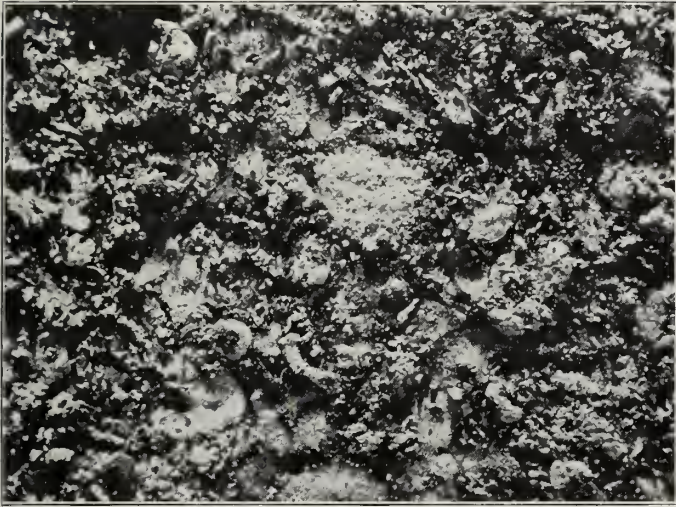
FIG. 4. Chester limestone. Maximum surface relief about 1 mm. Etching has removed the calcium carbonate cement and left the clayey, siliceous impurities of the stone as projections above the general surface. Disintegration of this specimen began after 4 repetitions of the soundness test, and complete failure resulted after 8 repetitions. The disintegration of the stone into a coarse sand showed that the bonding material was weak. (Magnification six times.)
