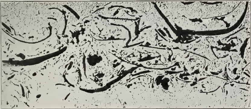
FIG. 5. Pennsylvanian limestone. Maximum surface relief about 1½ mm. This is a siliceous limestone containing fossils composed of calcium carbonate. These were dissolved during the etching and gave rise to the linear depressions. After 6 repetitions of the soundness test this specimen began to chip and split along the surfaces of fossils. After 11 repetitions, disintegration of the entire specimen was complete. This sample shows the type of results which may be expected in limestone with a localized porosity. (Magnification six times.)
