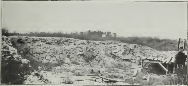
Fig. 6. General view of quarry in Area 3, illustrating the irregular surface of the limestone and the thin overburden.
