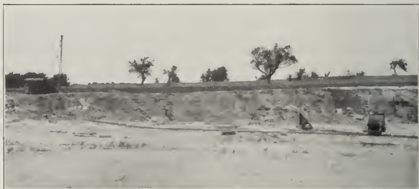
Fig. 5. General view of the quarry in Area 1, showing the almost flat-lying Pontiac limestone with a comparatively level surface and thin overburden.
