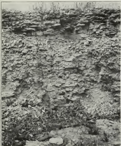
Fig. 4. Near view of the Pontiac limestone in quarry in Area 1, showing the fractured and thin bedded character of the stone.
