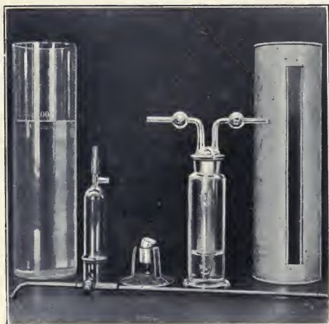
FIG. 3. — William Thomson calorimeter.
