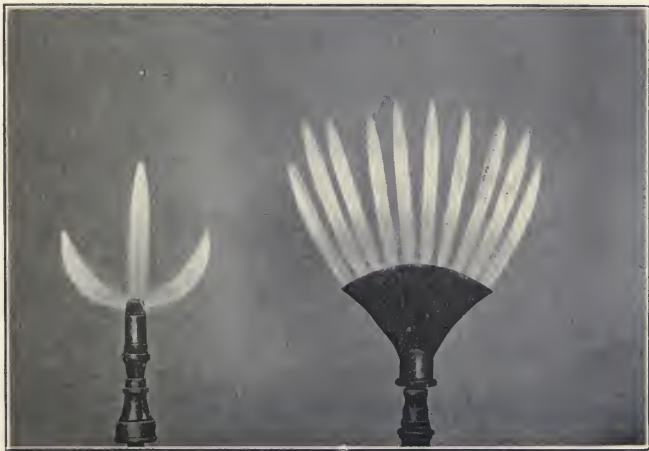
FIG. 26.—Cockspur and cockscorn burners.
