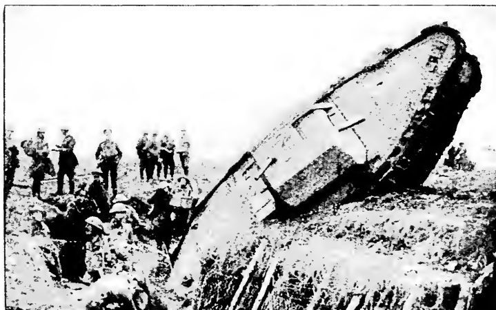
FAILURE OF A TANK TO CROSS A TRENCH
