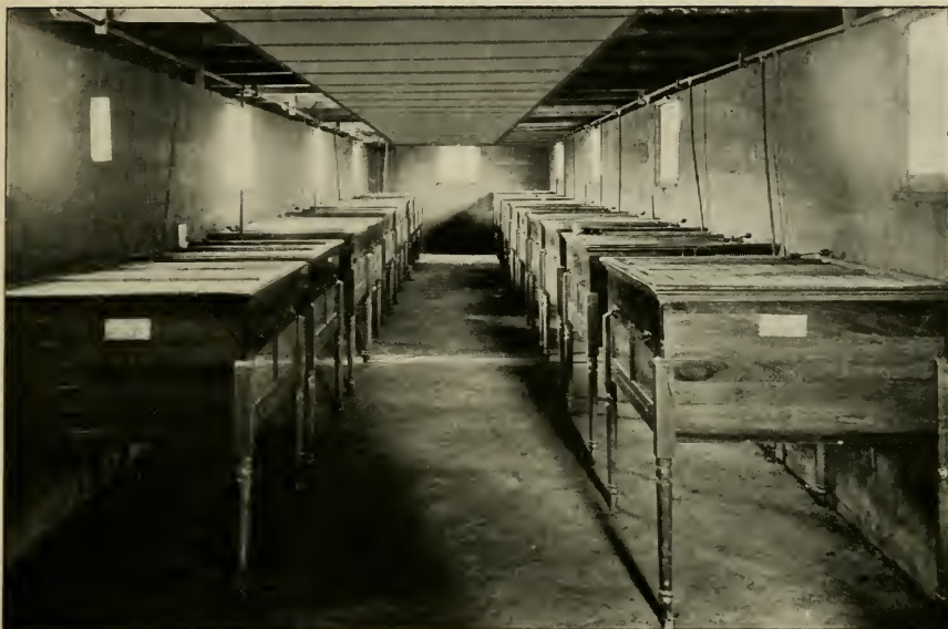
A corner in one of the incubator cellars. These machines are all heated by gas from a gas well on the farm.
